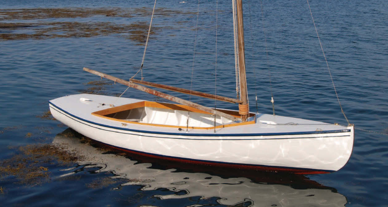
Royal Tern was restored in 2011 and went back into the water for the first time in years. In this photo, her mast is stepped forward of the cockpit. Since then, the mast step has been moved a bit farther aft.
