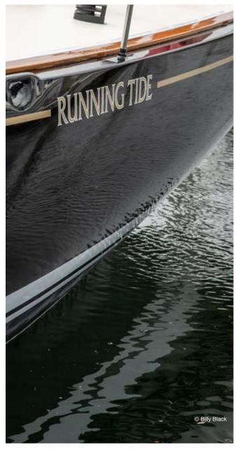
Over the next 18 months, the hull was taken down to bare aluminum and coated with ALEXSEAL®'s *Protective Primer 161*, re-faired, primed, and top coated in ALEXSEAL® *Premium Topcoat 501* in Super Jet Black. At the late June 2020 launch, the quality of the paintwork was visible to all.
